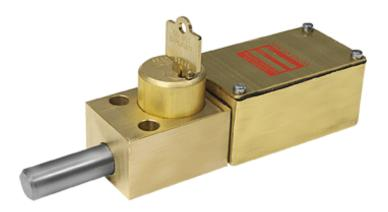
Type S auxiliary switches are slow-make, slow-break devices that respond directly to the movement of the lock bolt when the key is rotated. One, two, three or four sets of contacts are available. The Type S auxiliary switches can be furnished on the following interlocks:
